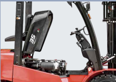
The wide-open hood, increasing maintenance space by 10%
